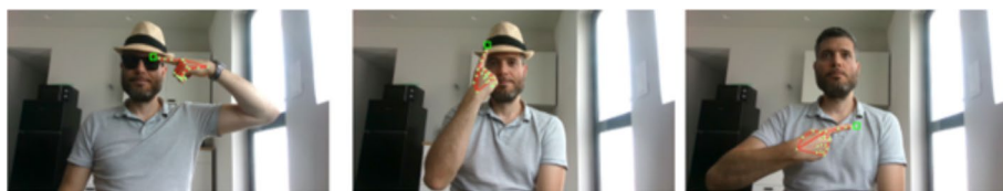
Fig. 3 Demonstration of the gesture tracking module, which accurately identifies index finger pointing across various directions and hand orientations. If a gesture remains spatially stable over consecutive frames, the module extracts pixel-space coordinates to generate a spatial prompt (see Section 4.1.2), which is then asynchronously forwarded to the segmentation module to define the Region of Interest (see Section 4.1.3)
