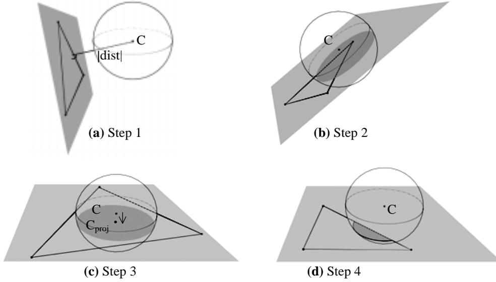
**Figure 3.** Sphere/triangle intersection test
