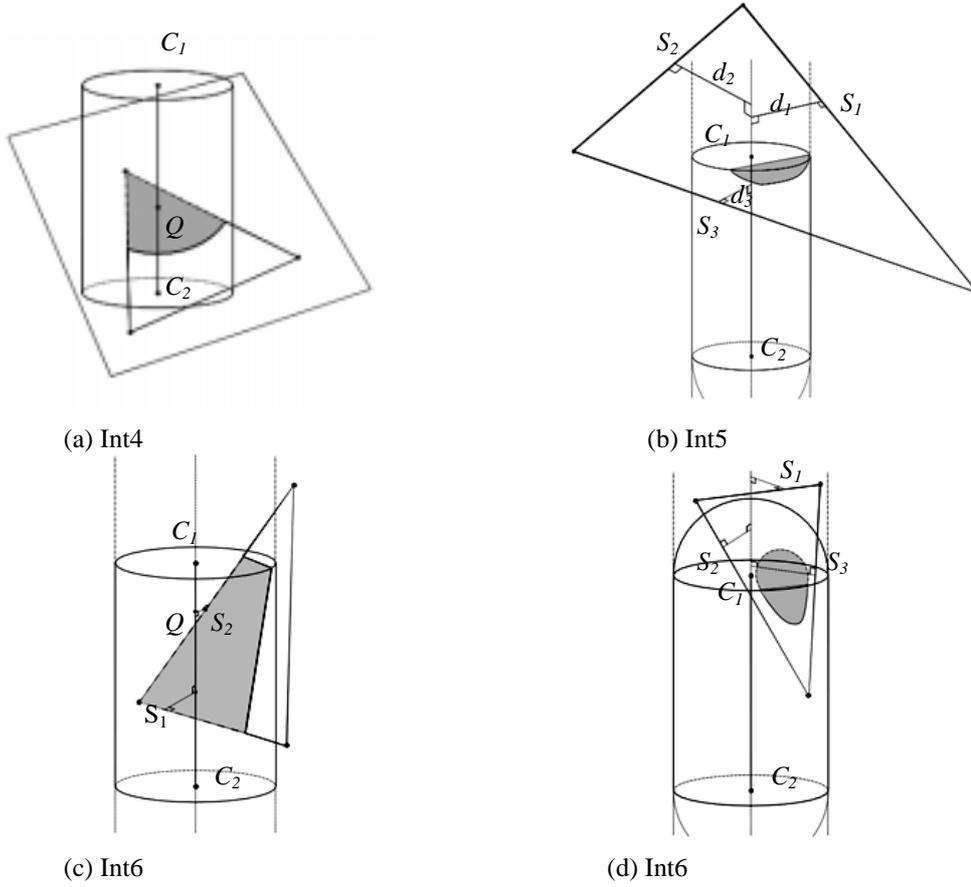
**Figure 6.** Cylinder/triangle intersection calculation, when the cylinder axis intersects with the triangle plane.
