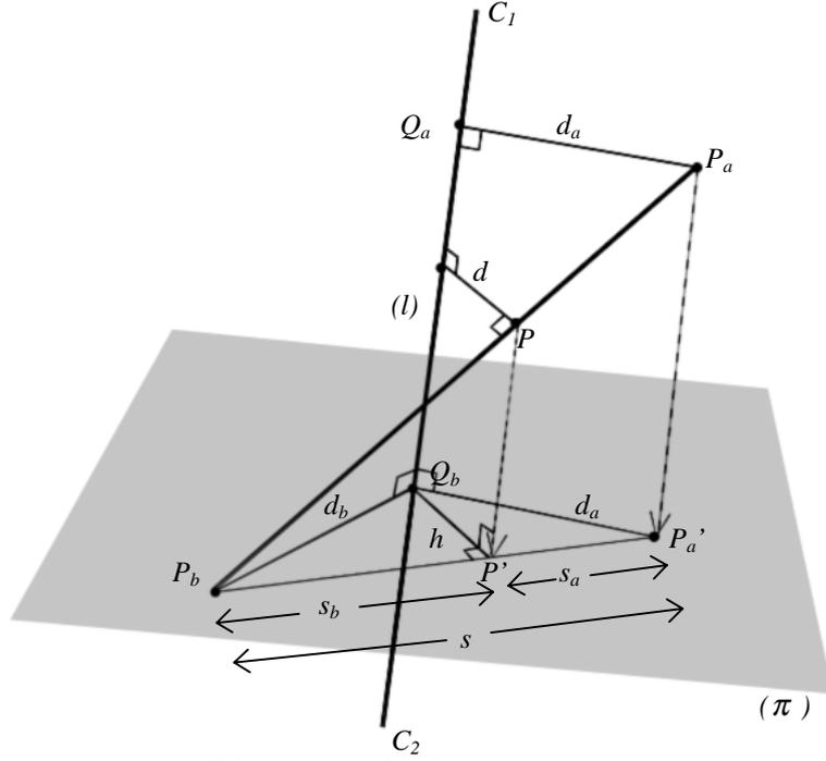
**Figure 7.** Calculation of the closest point  $P$  of segment  $P_aP_b$  to line  $(l)$ .
