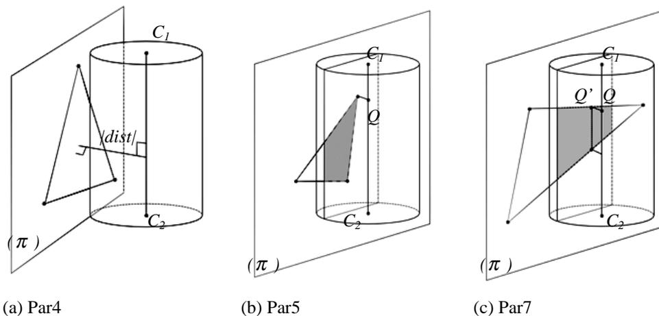
**Figure 5.** Cylinder/triangle intersection calculation, when the cylinder axis is parallel to the triangle plane.
