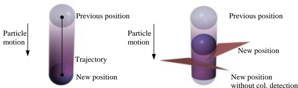
**Figure1.** Particle movement between 2 frames.
