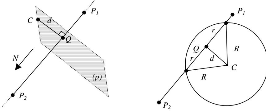
**Figure 4.** Line/sphere intersection.
