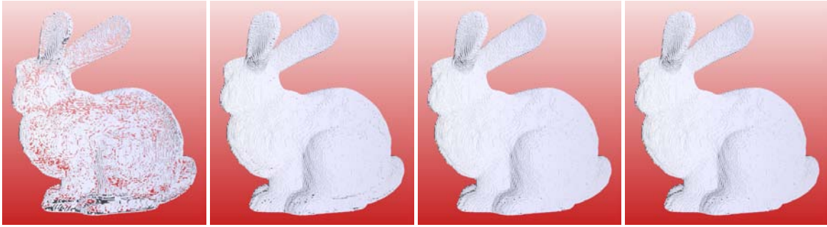
Figure 7: Comparison of the voxelization using the pixel shader clipping method at 256^3 volume resolution with 3, 6, 9 and 12 geometry shader vertices output. The number of voxels produced are 52382, 87690 and 89696 (complete voxelization) for 3, 6, 9 and above geometry shader output vertices, respectively.
